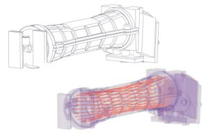
The detector is based on Tunable Diode Laser Absorption Spectroscopy (TDLAS) combined with a Herriot multipass cell to increase the lenght of the optical path and consequently the sensitivity of the detector. The advantage of TDLAS over other techniques for concentration measurement is its ability to achieve very low detection limits: LDL=100ppb.
