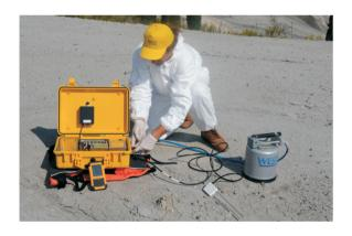
The power supply requirement of the TLDAS methane detector is very low: 2 Watt. It allows a very long operating time by using a single light and inexpensive NiMH battery.
