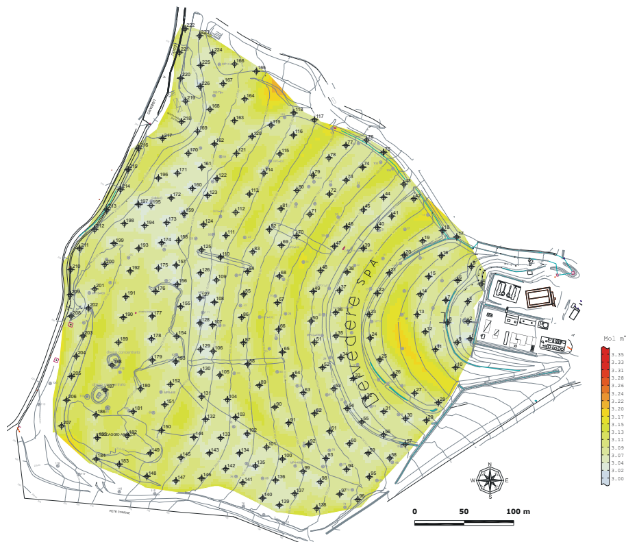
Figure 9. Standard deviation map associated to the isoflux map of LFG released from the cover of the MSW landfill. The black dots represent the locations of flux measurements performed with FLUX-meter.
