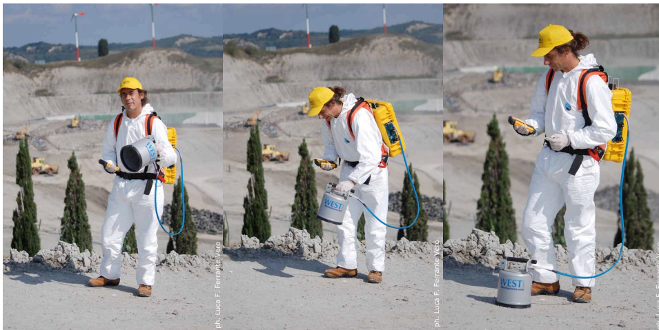
Figure 3. Steps of a field measurement with the FLUX-meter.
