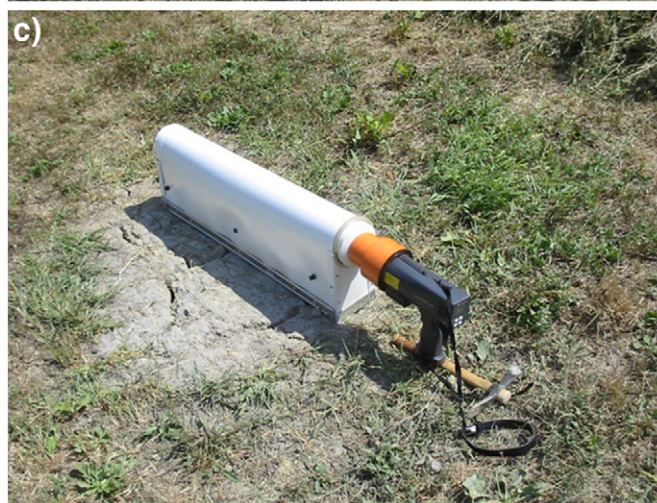
Fig. 2. Photos of the closed-chamber systems used in microseepage surveys in USA (a) and Europe (b, c). Methane concentration increase is measured by GC analysis of samples taken manually by syringes (a, b) or by direct detection by laser sensor (c).
