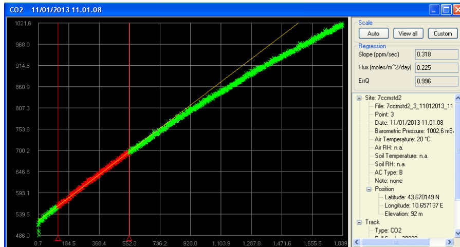
Figure 4. Graphical representation of the increasing concentration value vs time inside accumulation chamber.
