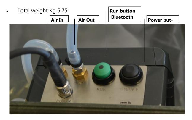
Snail micro flow air sampler @
